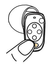
**To turn the hearing aids off:** Press and hold the button on the side of each hearing aid **for 6 seconds**. After 3 seconds, you'll hear the program change beeps—**KEEP PRESSING** until you hear a long beep, which signals the hearing aid is turning off.
