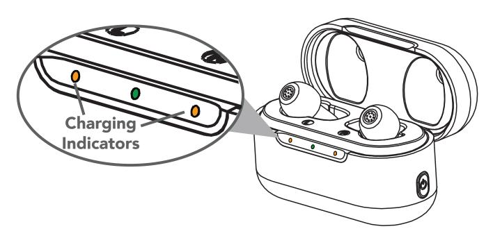
The case's hearing aid charging indicators illuminate orange while that side's hearing aid is charging. They turn green when the hearing aid is charged (and turn off after five minutes).
