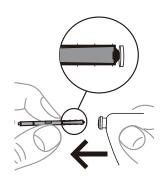
4. Pull the wax guard tool out of the stem. The new wax guard should stay in place. Discard the wax guard tool.
