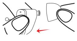
2. Pull gently on the dome to make sure it's secure. Then push the flaps of the dome back into place.
