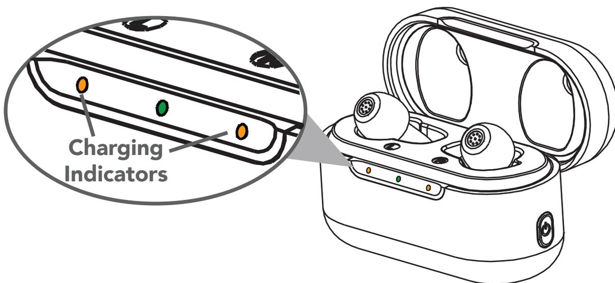
The case's hearing aid charging indicators illuminate orange while that side's hearing aid is charging. They turn green when the hearing aid is charged (and turn off after five minutes).
