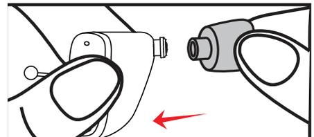
2. Pull gently on the dome to make sure it's secure. Then push the flaps of the dome back into place.
