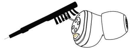
Remove the dome from each hearing aid's stem. Use the provided pick to clean the inside of the dome and around the stem. Clean the dome with a soft, moist cloth or mild soap and water. Make sure the dome is completely dry before you put it back on the stem.
