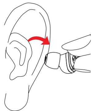
**To remove the dome:** Pull it off of the hearing aid's stem.
